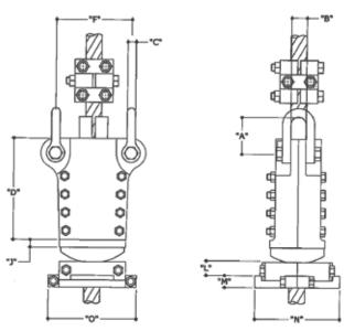
This gland has been developed from the "NU" type and has several features which make it particularly suited for the suspension of guide and rubbing ropes. The spherical seating enables the rope to be turned periodically to present fresh surfaces to the guide rope shoes and provides compensation adjustments for any uneven settlement of the headframe making vertical alignment of the rope in the gland easier.
