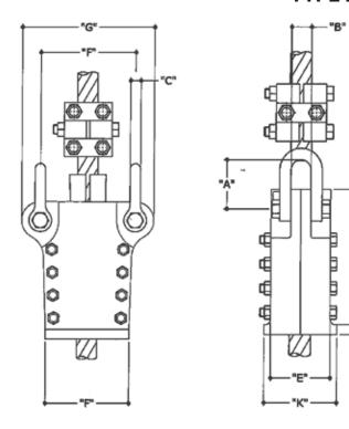
The NU gland is used for suspending guide or rubbing ropes in mine shafts, the base being supported on girders in the headframe or tower. It is also used for rope anchorage and the suspension of ropes during installation or maintenance.
