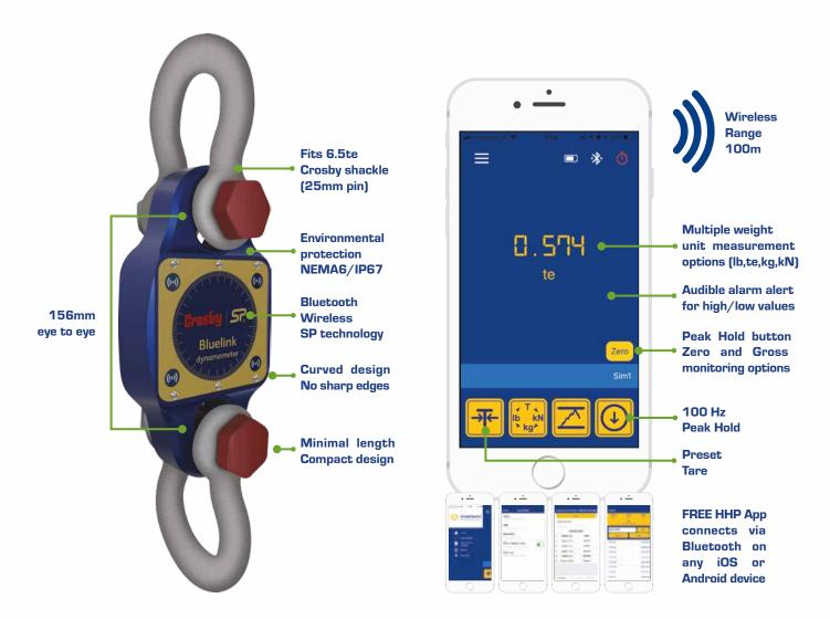
Designed to replace outdated mechanical products still in the field this 6500kg Dynamometer, the 'BlueLink' is the latest SP product to feature their proprietary Bluetooth wireless technology.
